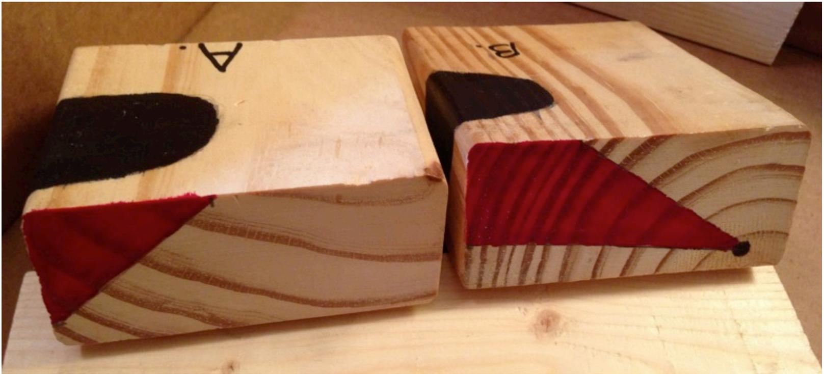
Knot “A” appears larger by its superficial extension on the piece of lumber, but Knot “B” actually DISPLACES more wood fiber. Therefore, Knot “B” is larger.
