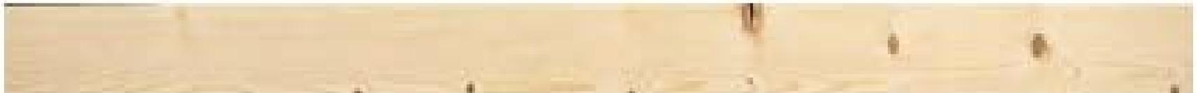
The Basic and Key Concept in the grading of Structural Lumber is the DISPLACEMENT of wood fiber by knots in any CROSS-SECTION.
