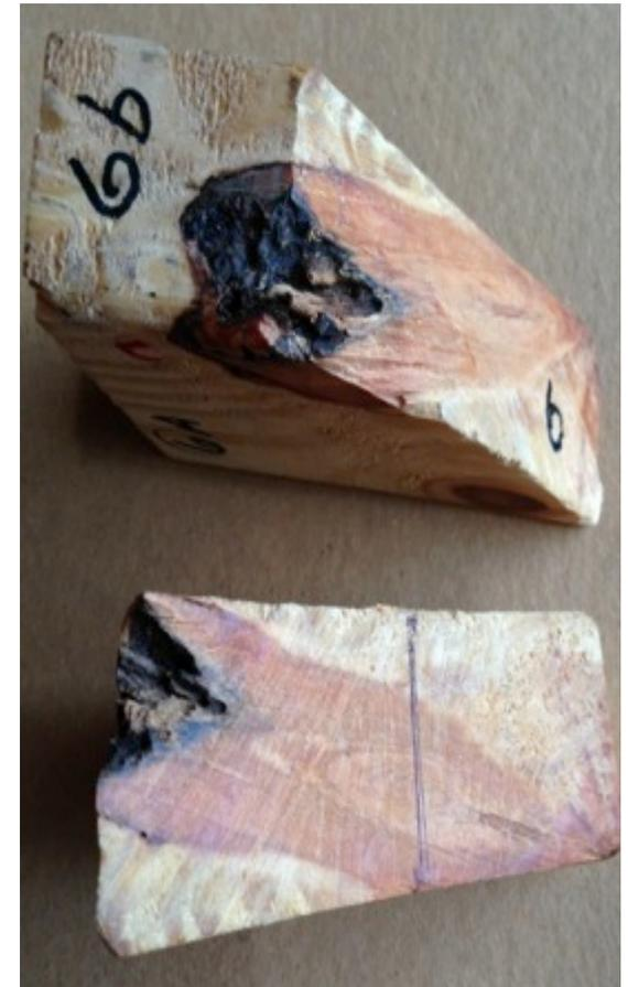
**Examples of two cross sections of two pieces of 2 x 10, showing two ugly knots in the superior piece and one not-so-ugly-knot occupying part of the face and edge in the lower piece.**
