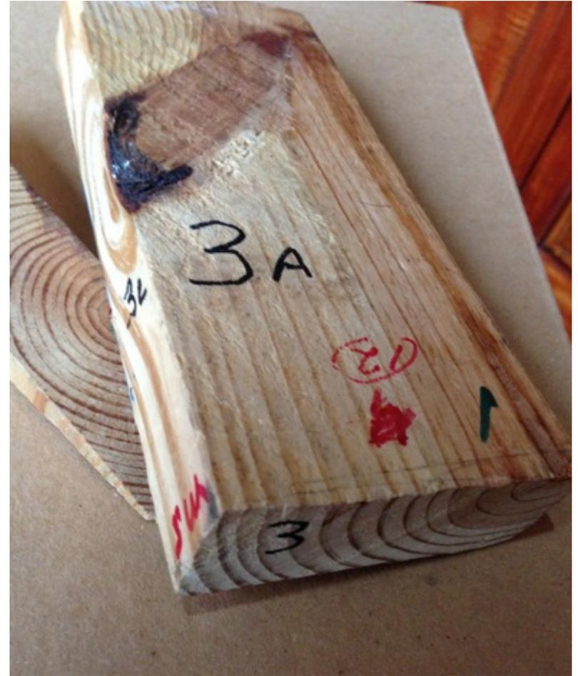
Note the evolution of the knot, from a “live-red” knot to a “dead knot” & later to a “decayed knot”.
