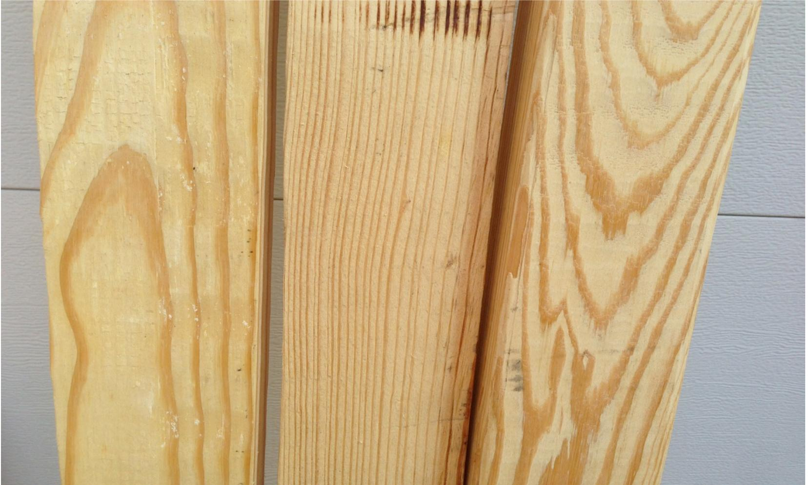
From Left to Right: Flat Grain (tangential) – Vertical Grain (radial) – Flat Grain
