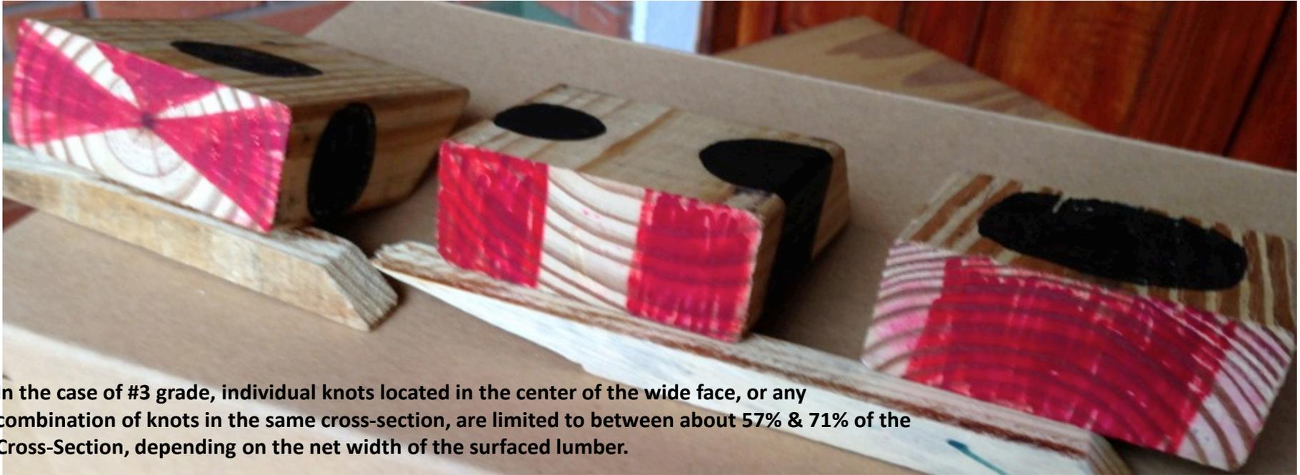
In the case of #3 grade, individual knots located in the center of the wide face, or any combination of knots in the same cross-section, are limited to between about 57% & 71% of the Cross-Section, depending on the net width of the surfaced lumber.
