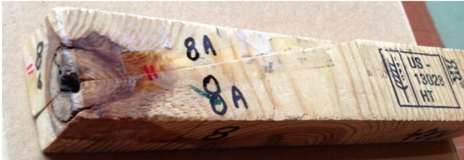
The same two pieces of 2 x 10 after having cut through the knots in the respective cross sections:
