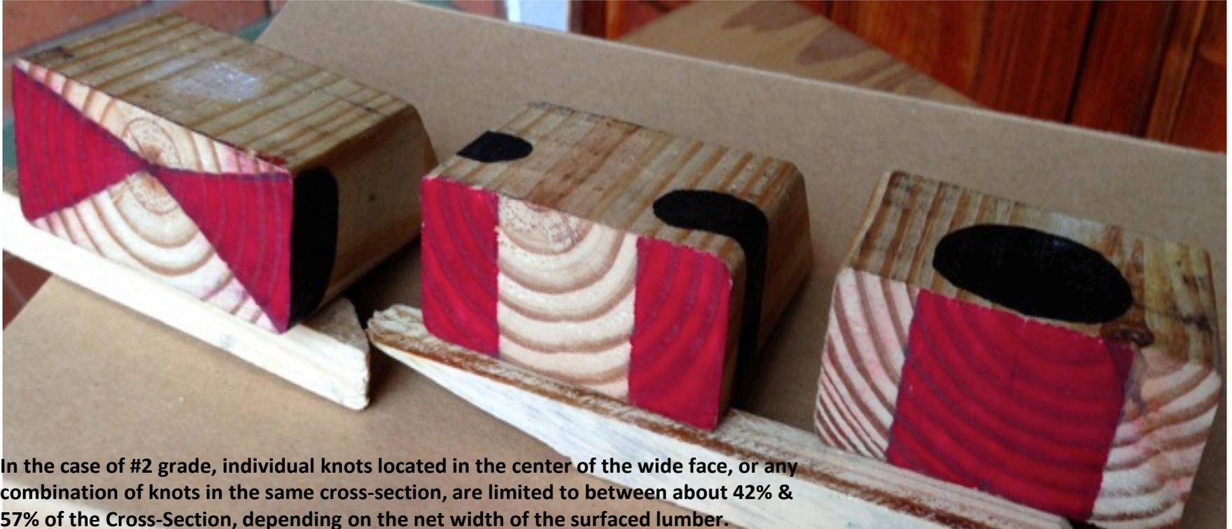
In the case of #2 grade, individual knots located in the center of the wide face, or any combination of knots in the same cross-section, are limited to between about 42% & 57% of the Cross-Section, depending on the net width of the surfaced lumber.
