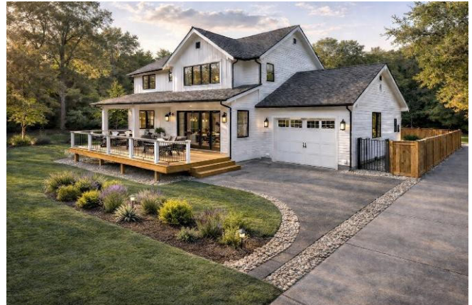
Figure 6. Before-and-after representation of a single-family house that implemented Zone 0. Note the relocation of the plants away from the deck and the installation of a noncombustible gate. While not required, it is best practice to install metal screening around the deck base to keep embers and debris out. Once Zone 0 is finalized, the guidance document will provide tips and tricks for addressing issues like this.
