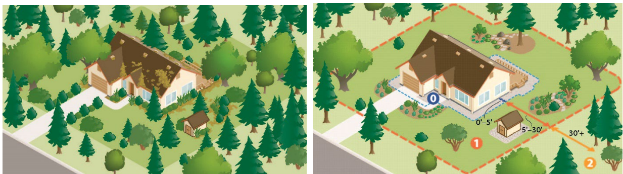
Figure 2: This is an illustrative example of the defensible space actions taken before and after using the three defensible space zones. Zone 0 applies to all structures. In the after instance (on the right), the pathways for fire to travel have been disconnected between planting groups or islands of landscaping. Additionally, the lower branches of trees have been removed to prevent fire from traveling through the treetops. Zone 0 actions eliminate the potential for embers to ignite combustibles adjacent to the structure.
