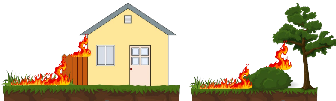
Figure 8: The left image illustrates how fire can progress through the vegetation to the fence and from the fence to the structure. Installing a metal or noncombustible panel or gate can prevent the transmission of fire to the structure. This process is very similar to the role that shorter vegetation plays, where it can act like a “fuel ladder” and assist fire in climbing into the canopy of the taller vegetation shown as a tree in this example. Image courtesy of the UC ANR Fire Network.
