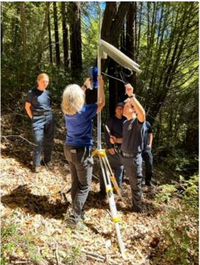
CAL FIRE and staff from N5 Sensors install remote sensing technology at JDSF. These tests will help determine if the sensors would be a viable solution to complement the ALERT Wildfire camera network for early detection and observation of fires and other potentially hazardous conditions.
