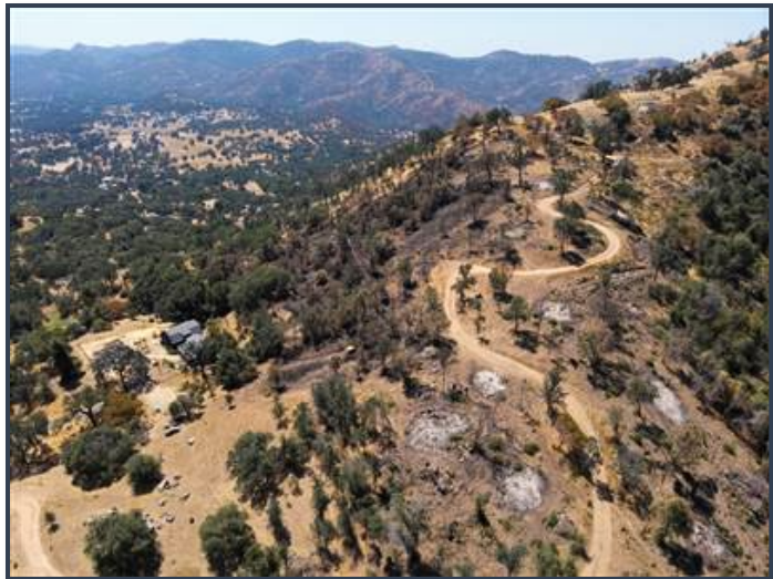
Figure 1. View of where the fire was stopped by the fuel break. Fuel break extended 200' on both sides of road. The white spots are brush piles burned Spring 2023.
