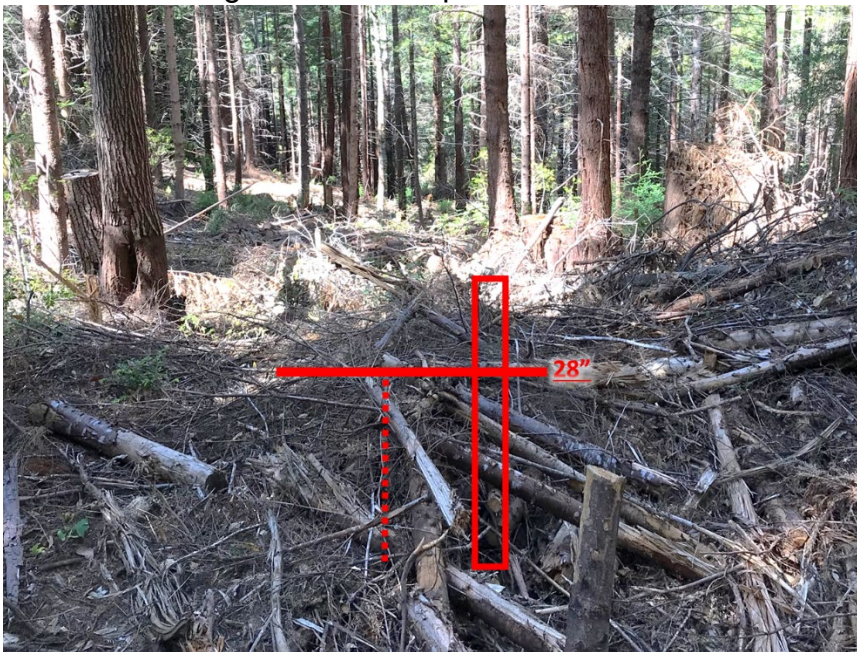
Figure 32: Example of harvest slash depth measurement; from the soil surface to the highest point where slash sticks up, is the slash depth.
