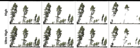
Figure 2. Subsets of filtered UAS-structures from motion (SM) point clouds (15 m × 30 m) for the 20 combinations of the build dense cloud Quality and depth map filter parameter settings.
