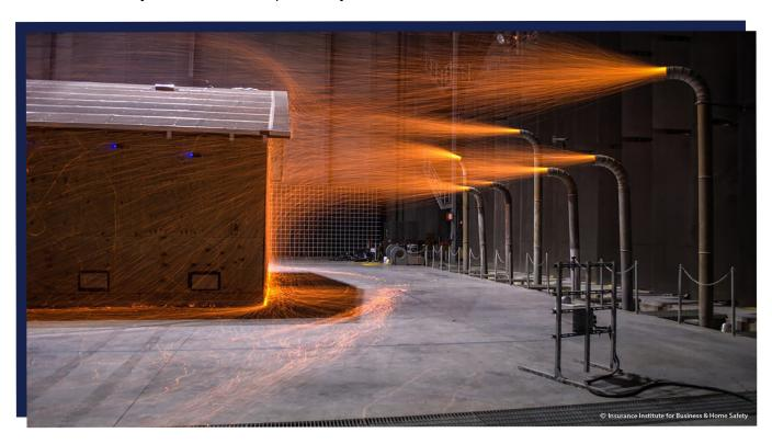
As part of its effort to reduce wildfire-caused building ignitions in vulnerable communities, IBHS Research Center developed the ability to simulate ember exposure on building components to better understand how structures ignite.
