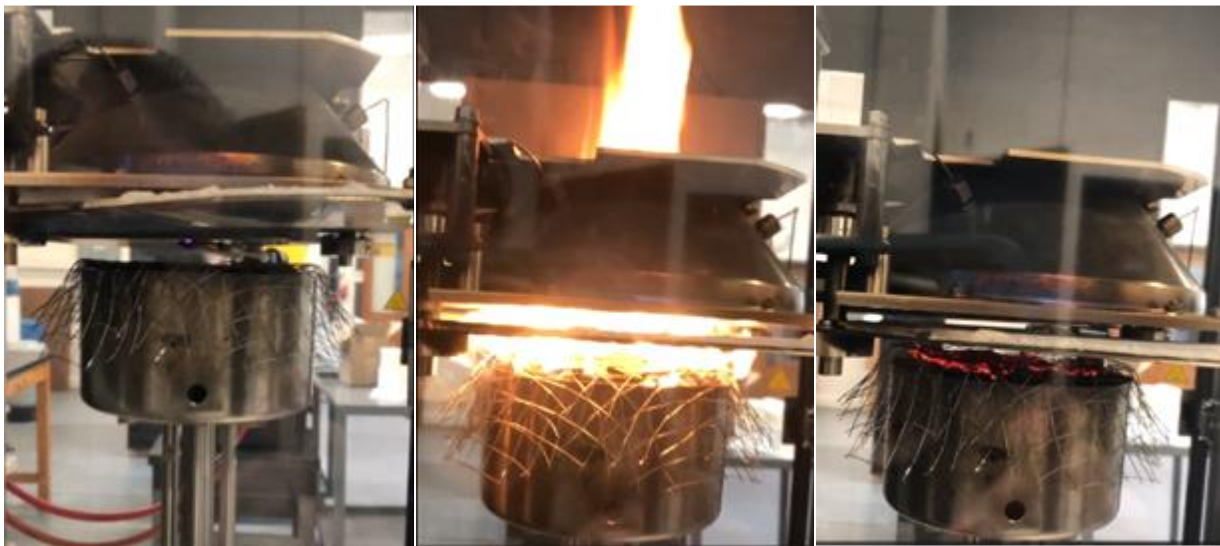
Figure X. Cone calorimeter test apparatus for measuring plant flammability. Photo 1 shows the small plant parts being preheated. Photo 2 shows ignition has occurred and the small plant parts consuming. Photo 3, small parts have been consumed that the plant parts are in the final, glowing stage of consumption
