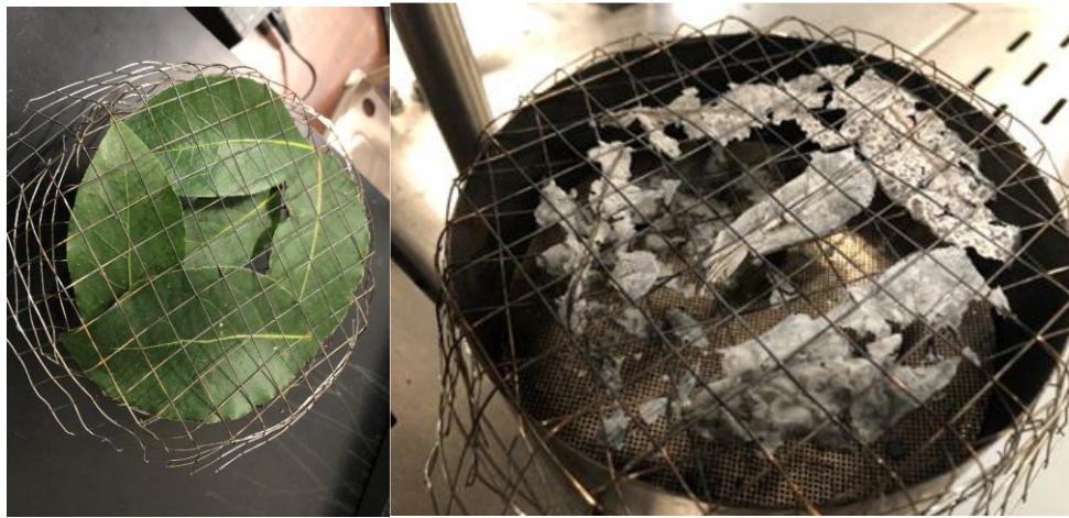
Figure 6.1. Photo 1, small plant sample prepared for burning in a cone calorimeter. Slide 2, same sample post-burn. Figure shows the burning process.
