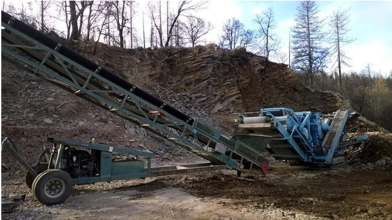
Figure 11. Rock crusher operating at the BMDSF quarry site.
