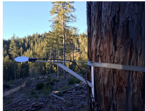
Figure 9: Photograph of leaf wetness sensor (LWS) secured to a bracket and mounted at a height of 6.1 meters (20 feet) in a S. sempervirens tree at the harvested ridge study site.
