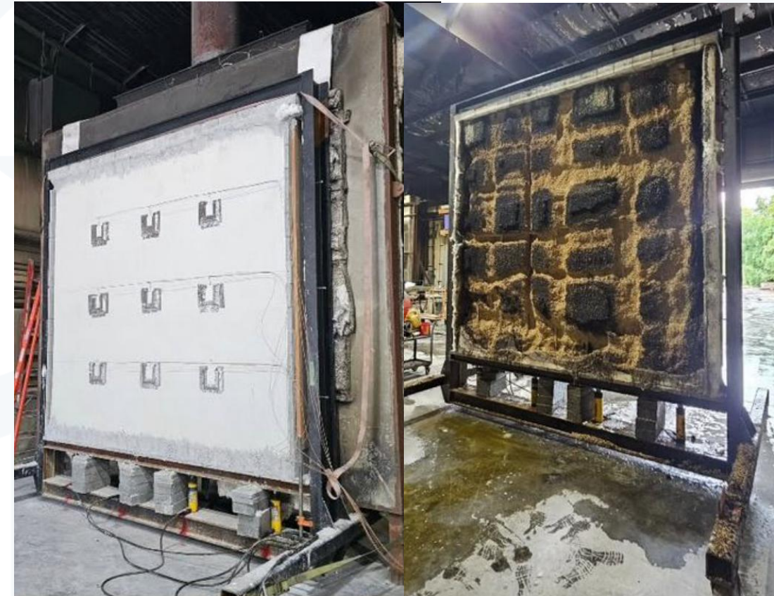
Hempcrete ASTM E119 Fire Test – Intertek Facility in York, PA (2024)
