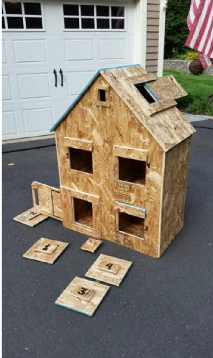
At this point, you should have plenty of scrap 7/16" plywood around. Before you start throwing it in the scrap pile, you will need to create two (2) covers in order to control smoke and fire gases through interior openings. Covers are needed for the following openings: 8x8" wall opening between lower rooms, 8x8" ceiling opening between first and second floor.
