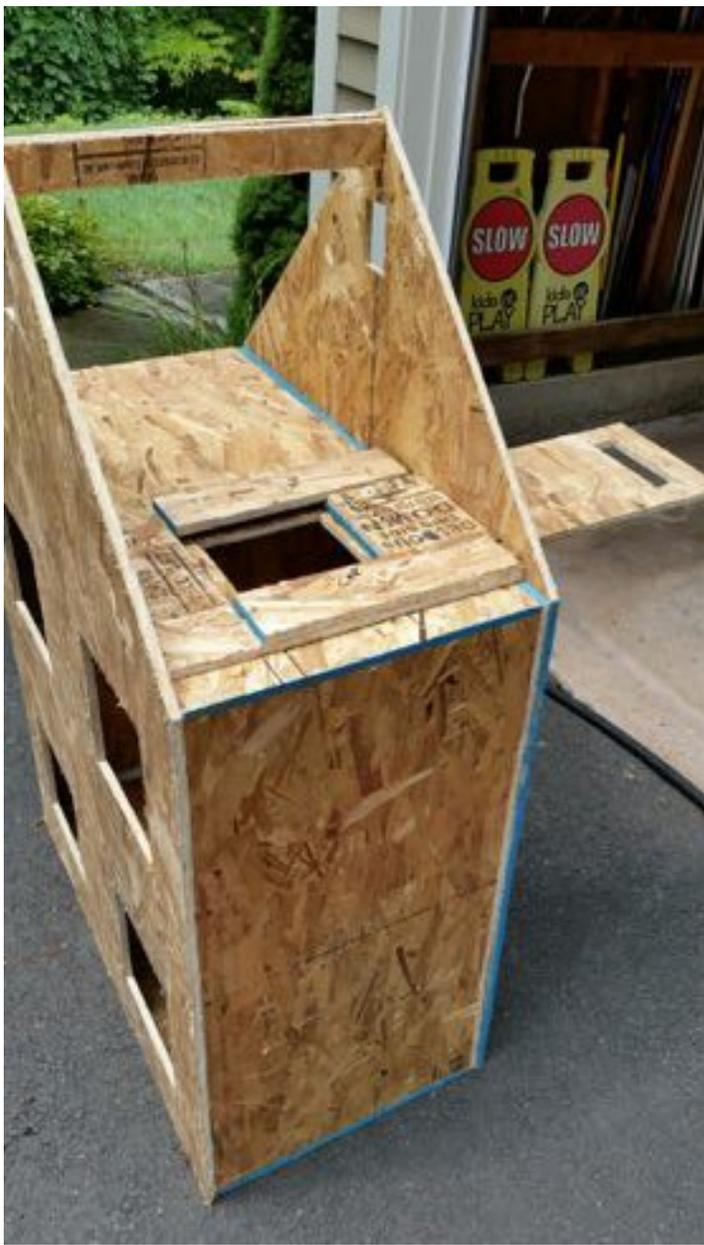
At this point, your assembled doll house should look similar to the photo on the left. Before you go any further, you will need to install plywood cleats and create a guide for the sliding ceiling cover. This is best accomplished by cutting strips of 1" and 2" OSB. Be sure to cut extra strips of 1" and 2" OSB as you will be repeating this process for the roof vent slide and the front door vent slides. The ridge pole shown in the picture is optional and not necessary for roof panel installation.
