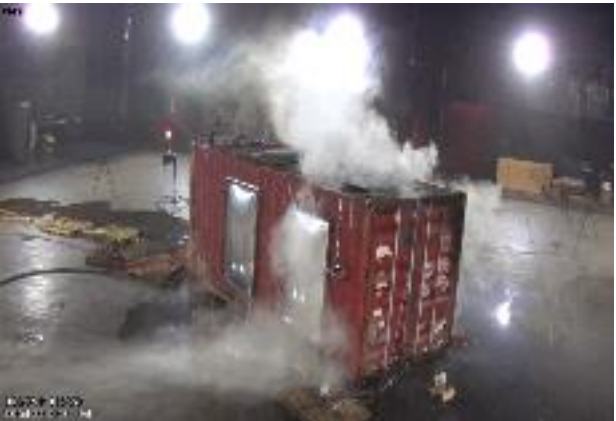
TR propagation after water flow off [TR + 01:13:05]
