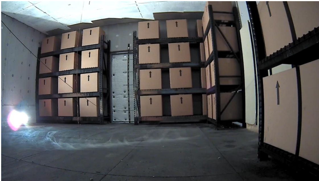
Interior view, 16 minutes of TR & gas accumulation before ignition
