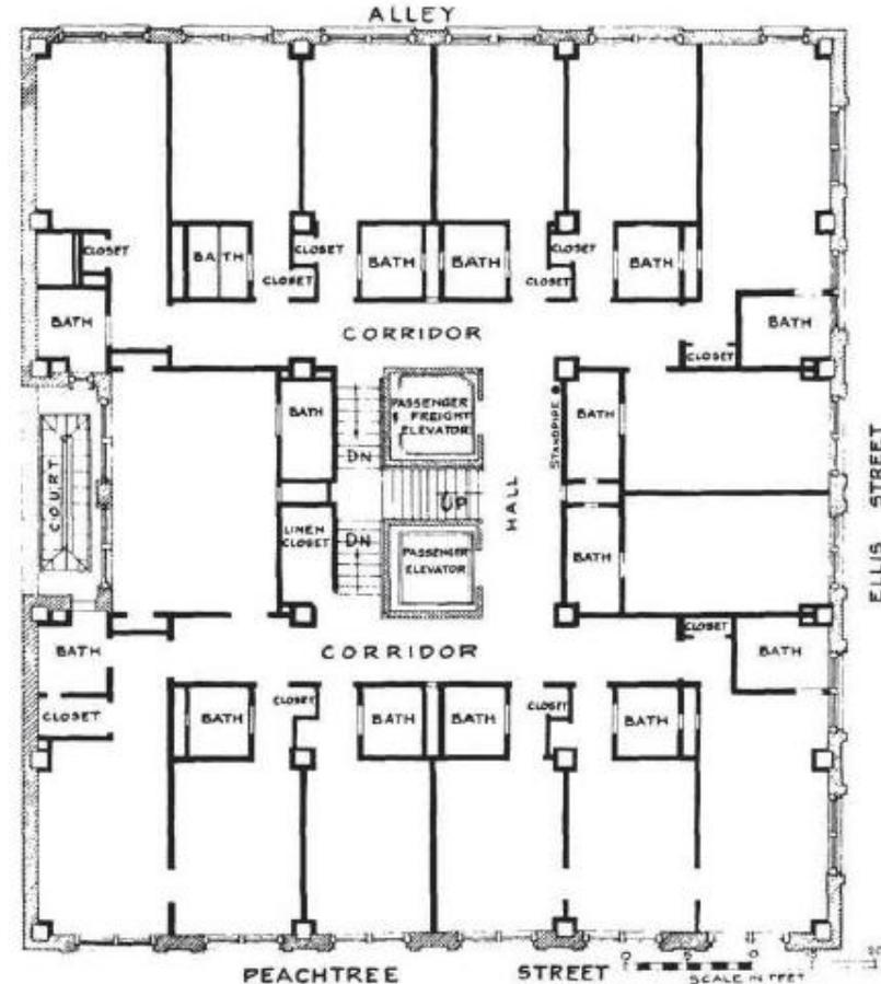
Plan of the third floor. The fire is supposed to have started near the end of the corridor, upper left in this plan, although the exact origin may never be known. The arrangement was the same on all floors above.
