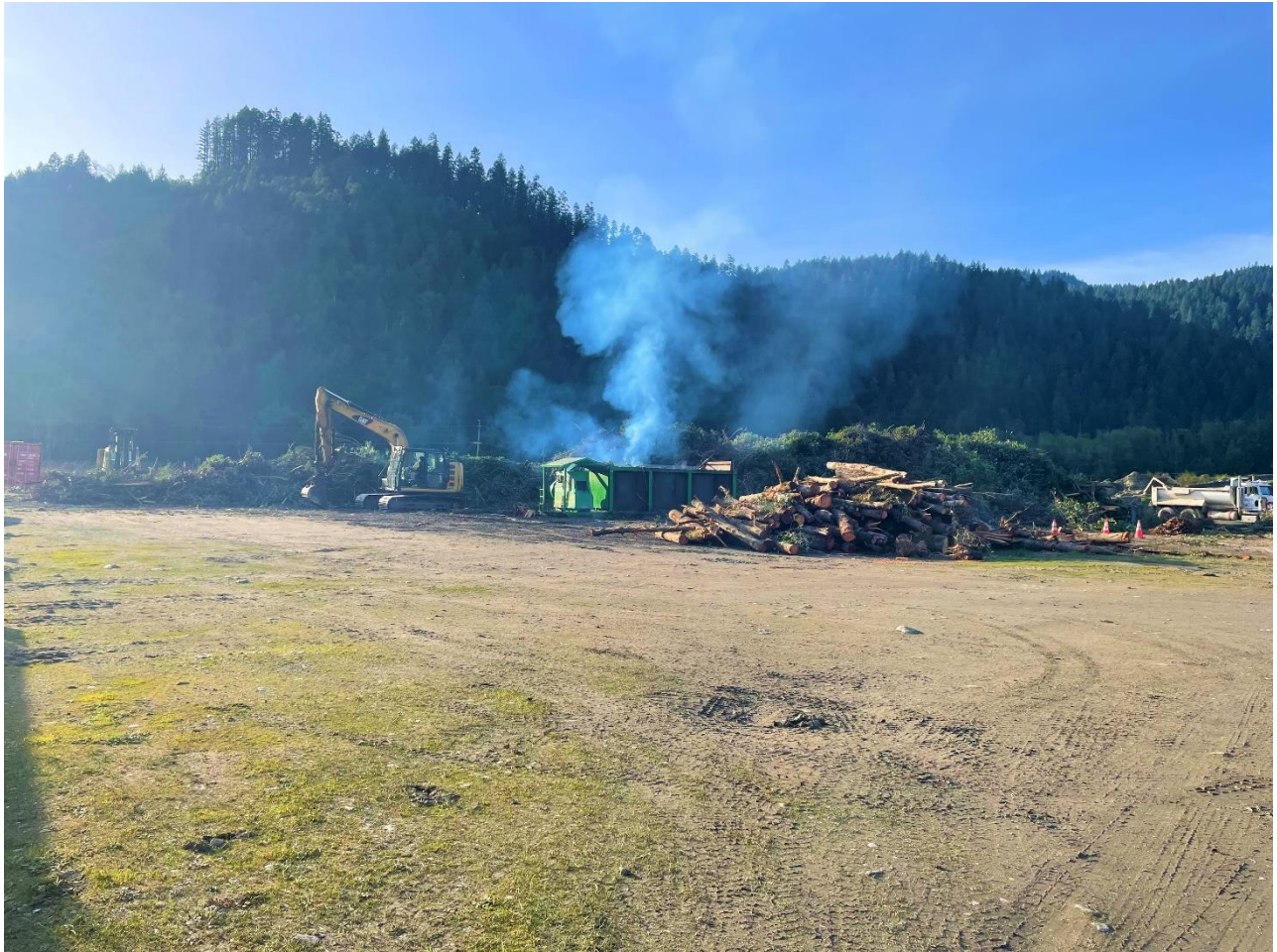
Image 12 Air Curtain Burner being utilized for storm damage clean-up in Willow Creek.
