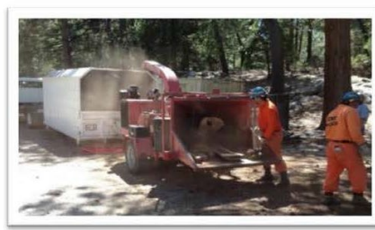
Camp Crews Chipping Infested Wood
