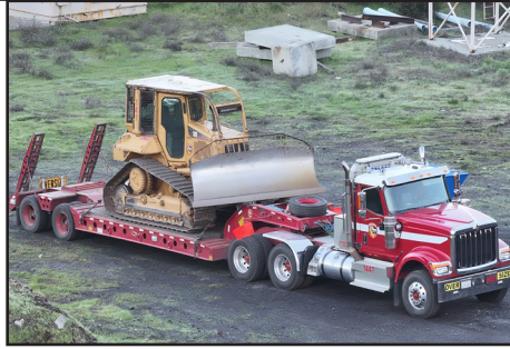
CAL FIRE Dozer & Transport Trailer
