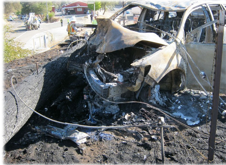
Vehicles contacting Power poles cause ignitions
