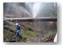
Pre-tested pipe must be pressure tested to a minimum of 125% of the maximum operating pressure for 4 continuous hours.
